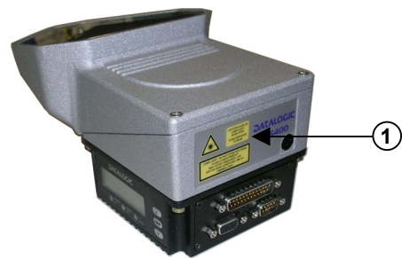
Figure B ① Warning and Device Class Label
